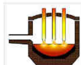
A schematic cross-section through an EAF. Three electrodes (yellow), molten bath (gold), tapping spout at left, refractory brick movable roof, brick shell, and a refractory-lined bowl-shaped hearth.
